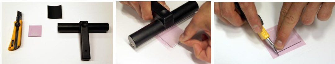
Figs. 55–57. Preparation of materials. From left: a set of basic tools, the process of applying a sheet of photopolymer material to a glass base, trimming the excess film to the desired size.
